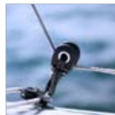
Cheek plates twist to open block
