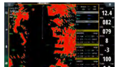
A faster rotation speed allows a faster refresh of targets in the PPI (radar screen).
